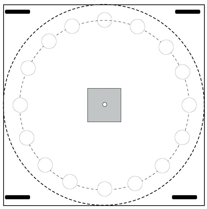
take 1- 24 inch x 24 - 1/2 "thick plywood draw a circle 20.25 inches in diameter drill 16 2" holes into plywood spaced equally apart around the circle (16 golf balls 1.68 inches in diameter dropped into 1.75-2 "holes) draw a second circle 24 " in diameter and cut outside off with jigsaw drill a 1/2 "hole in middle
